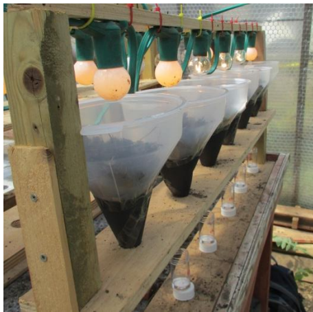
Figure 7: Tullgren Funnels with soil cores running through. The black card helped ensure the invertebrates moved downwards into the collection pots containing 70% ethanol. E. Rendells, 2014
