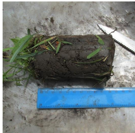
Figure 8: A soil core being prepared for running through a Tullgren funnel. The vegetation is removed and the top 10cm of the core are cut off and broken into regular sizes for the funnels. E. Rendells, 2014
